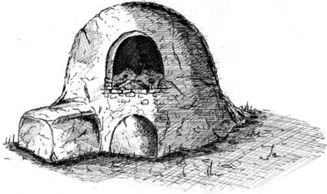
Figure 4: a beehive oven made of clay in the courtyard of a house in Peru. Drawing based on a photograph in The Cook's Room. The ledge on the left is a working platform, the stone door is propped up in the front.
